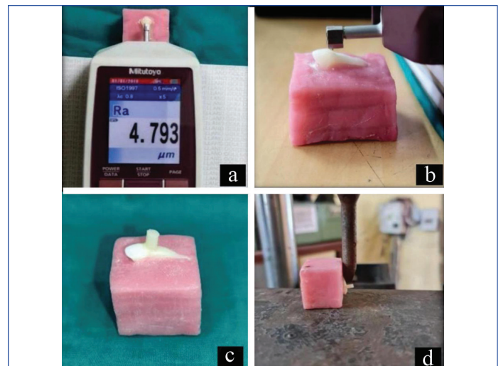
[Table/Fig-2]: a) Surface roughness measured by a digital surface profilometer; b) Magnified view of (a); c) Specimen ready for shear bond strength measurement; d) Shear bond strength of the specimen measured by Universal Testing Machine.
